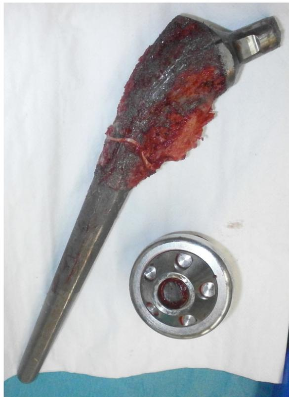
**Fig. (1b).** Detail of neck fracture of femoral component.
