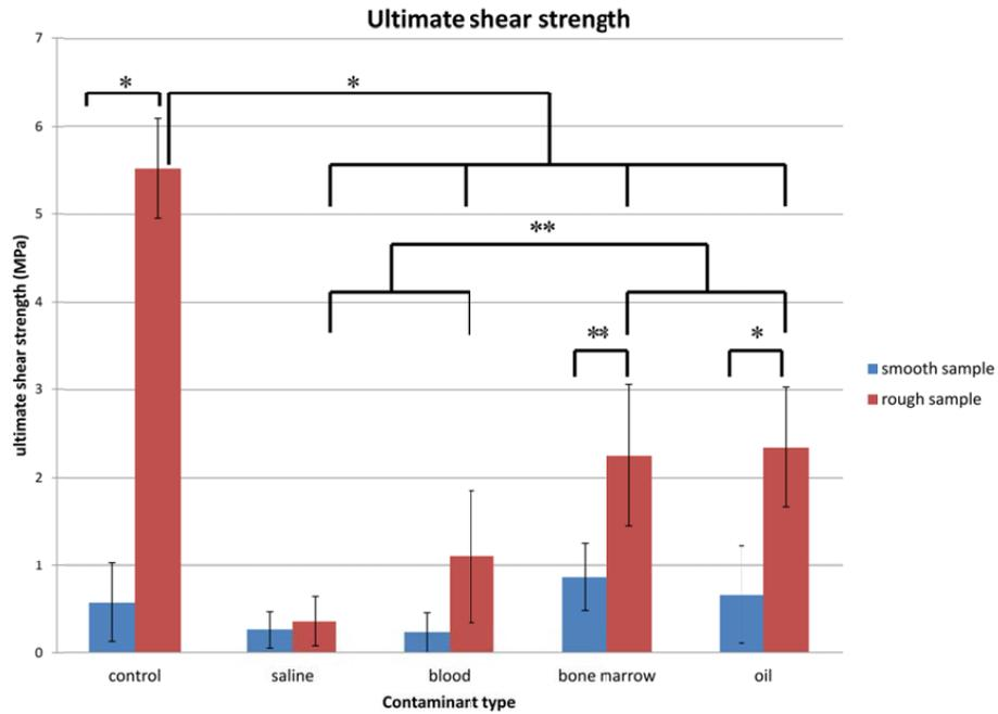
Fig. (1). The ultimate shear strength for each surface preparation, error bars represent standard deviation, \*= p<0.001, \*\*= p<0.05.
