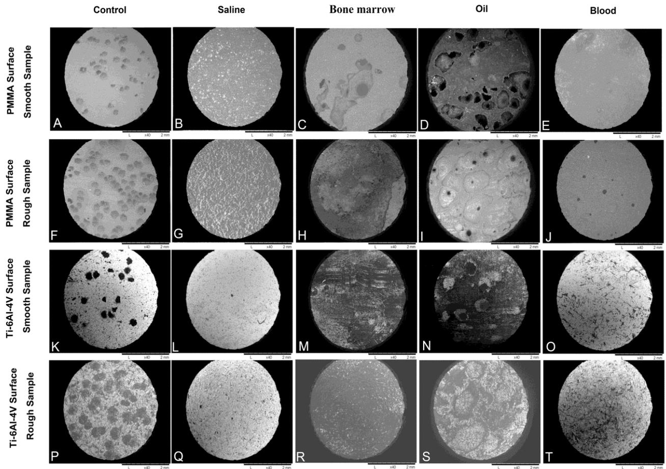
**Fig. (3).** 40x magnification SEM images of PMMA surface and dowel surface. (A-E) PMMA surface of each smooth sample group; (F-J) PMMA surface of each rough sample group; (K-O) Ti-6Al-4V dowel surface of each smooth sample group; (P-T) Ti-6Al-4V dowel surface of each rough sample group.
