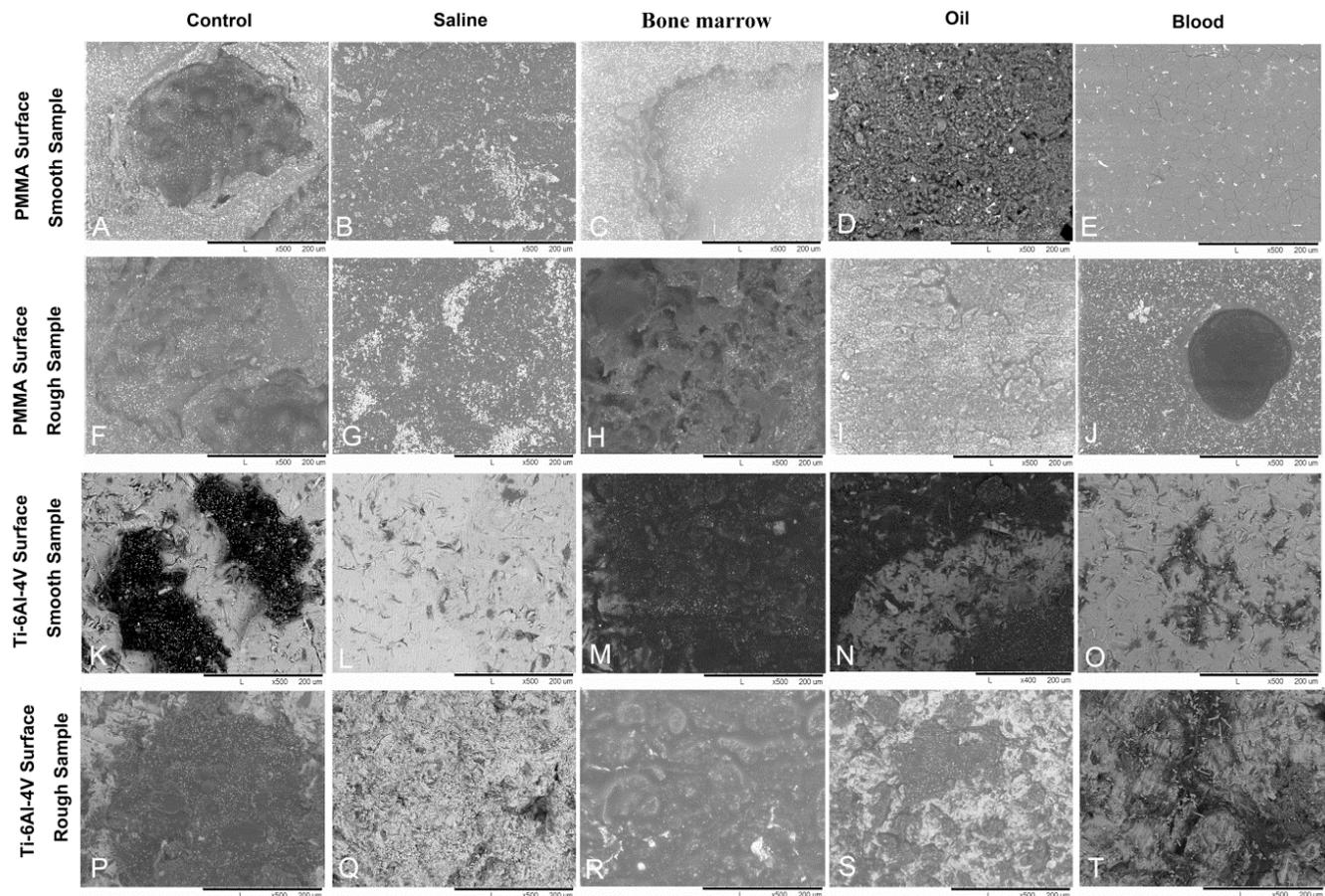
**Fig. (4).** 500x magnification SEM images of PMMA and dowel surfaces. (A-E) PMMA surface of each smooth sample group; (F-J) PMMA surface of each rough sample group; (K-O) Ti-6Al-4V dowel surface of each smooth sample group; (P-T) Ti-6Al-4V dowel surface of each rough sample group.
