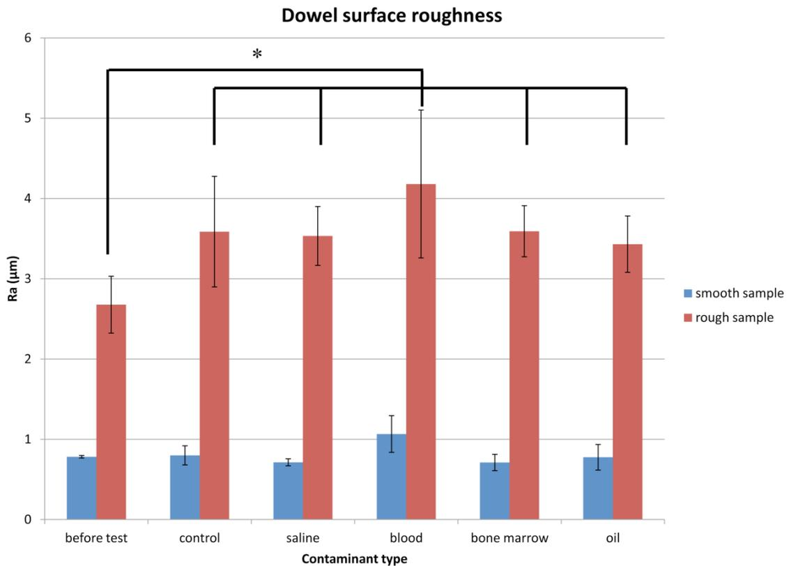
Fig. (2). The Ra for each surface preparation for different bodily contaminants, error bars represent standard deviation., \*= p<0.001.
